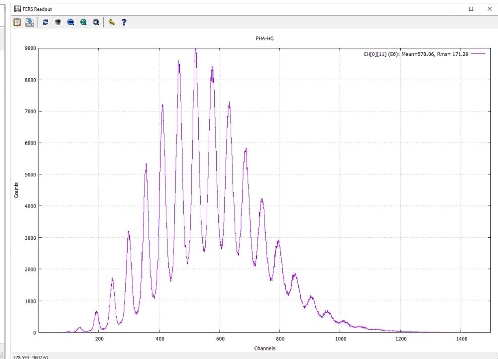
SiPM pulse height spectrum with the clearly visible photopeaks
