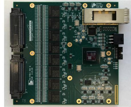
We also performed magnet field test (1.5T), but saw no effect to components (incl optical Tx/Rx)
