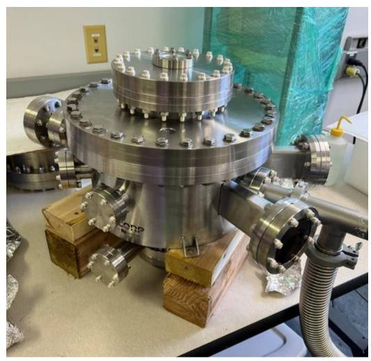
Scattering chamber delivered and leak checked.
