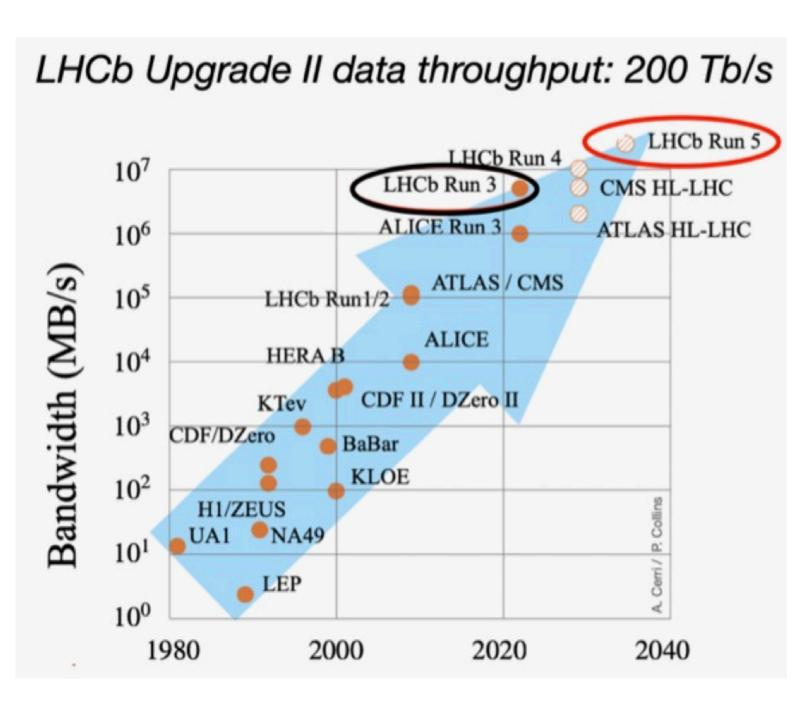
LHCb Upgrade II will produce highest bandwidth of any LHC experiment
