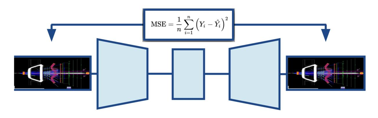
The performance is checked with reco vs original pulse shape on a 100 GeV sample (that was not used for training) → perfect reconstruction of the full pulse shape from 4 floats
