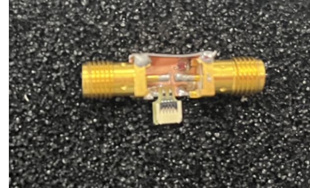
Probe connected to SMA (PROBE)
