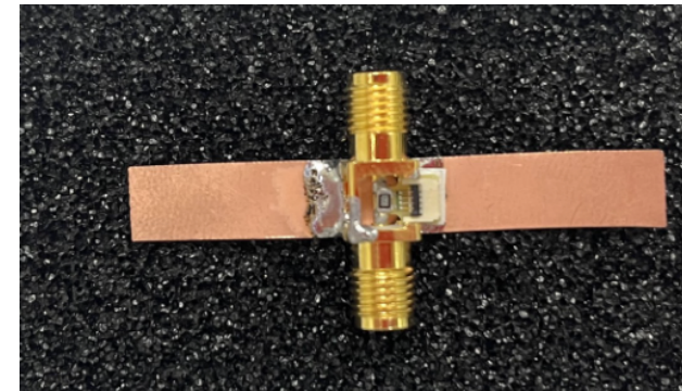
Probe connected to SMA with 100 ohms in between P and N of output (PROBE + 100 ohms)
