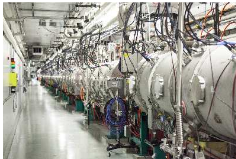
Layout of Linac RF with NC and SRF Modules
