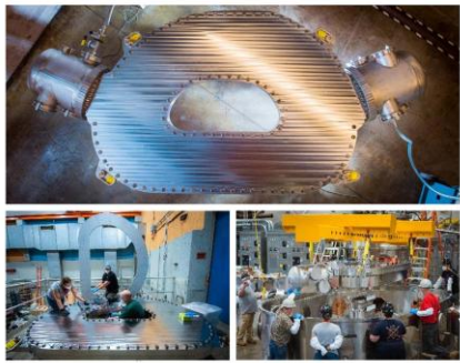
The TFMC is a large scale 20 T no-insulation REBCO magnet
