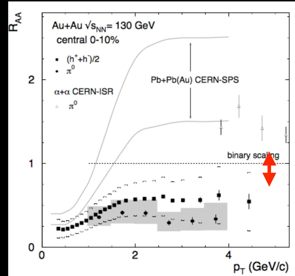
Suppression of high- $p_T$  particle production vs pp: **Jet Quenching**
