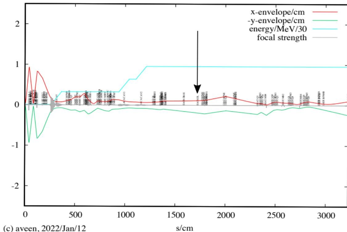
Typical 2 RMS e-Linac beam envelope. Radius of beampipe is 2.5 cm.
