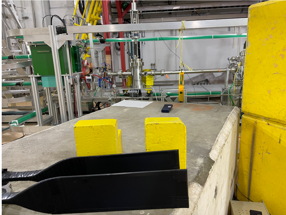
Figure 2: View of current test setup looking from behind the two scintillator bars, through the lead collimators, to the target chamber.
