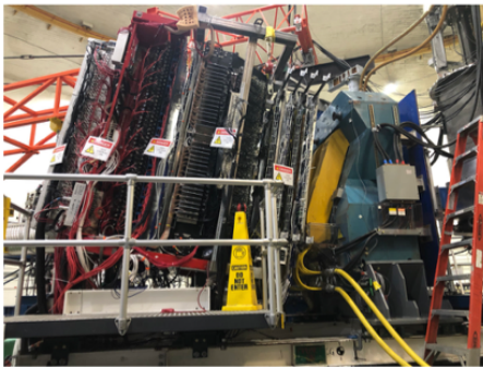
Cabling up the calorimeter, front end electronics, and DAQ in the hall
