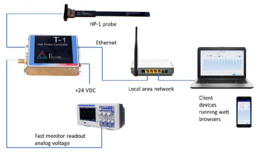
It is possible to use the Hall probe to provide feedback to control the power supply, but probably not necessary in our case.
