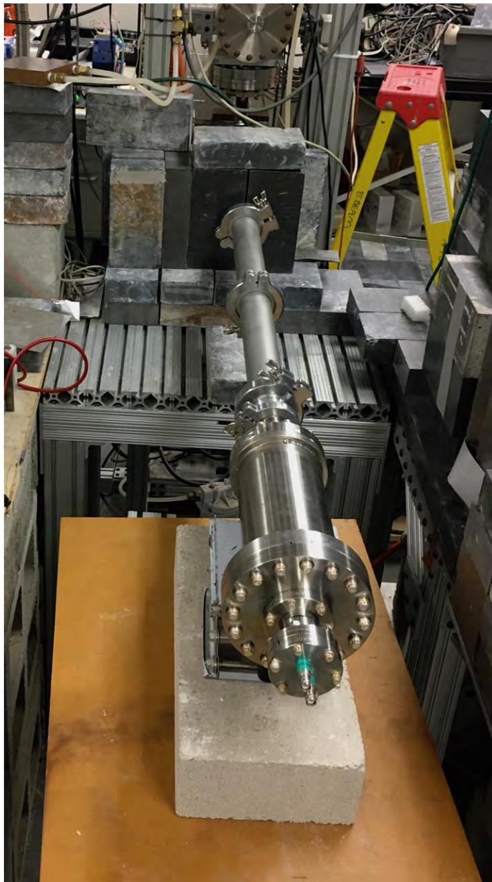
**Figure 4-61:** The Faraday Cup, installed directly on the beamline.
