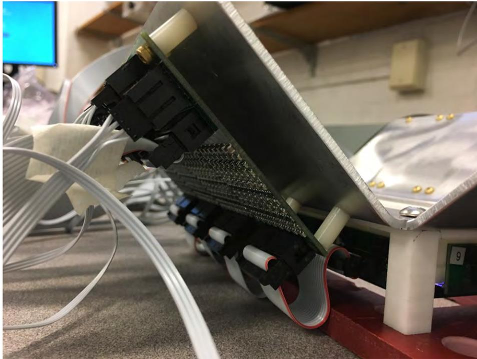
**Figure 4-45:** Closeup of the focal plane detector support structure.
