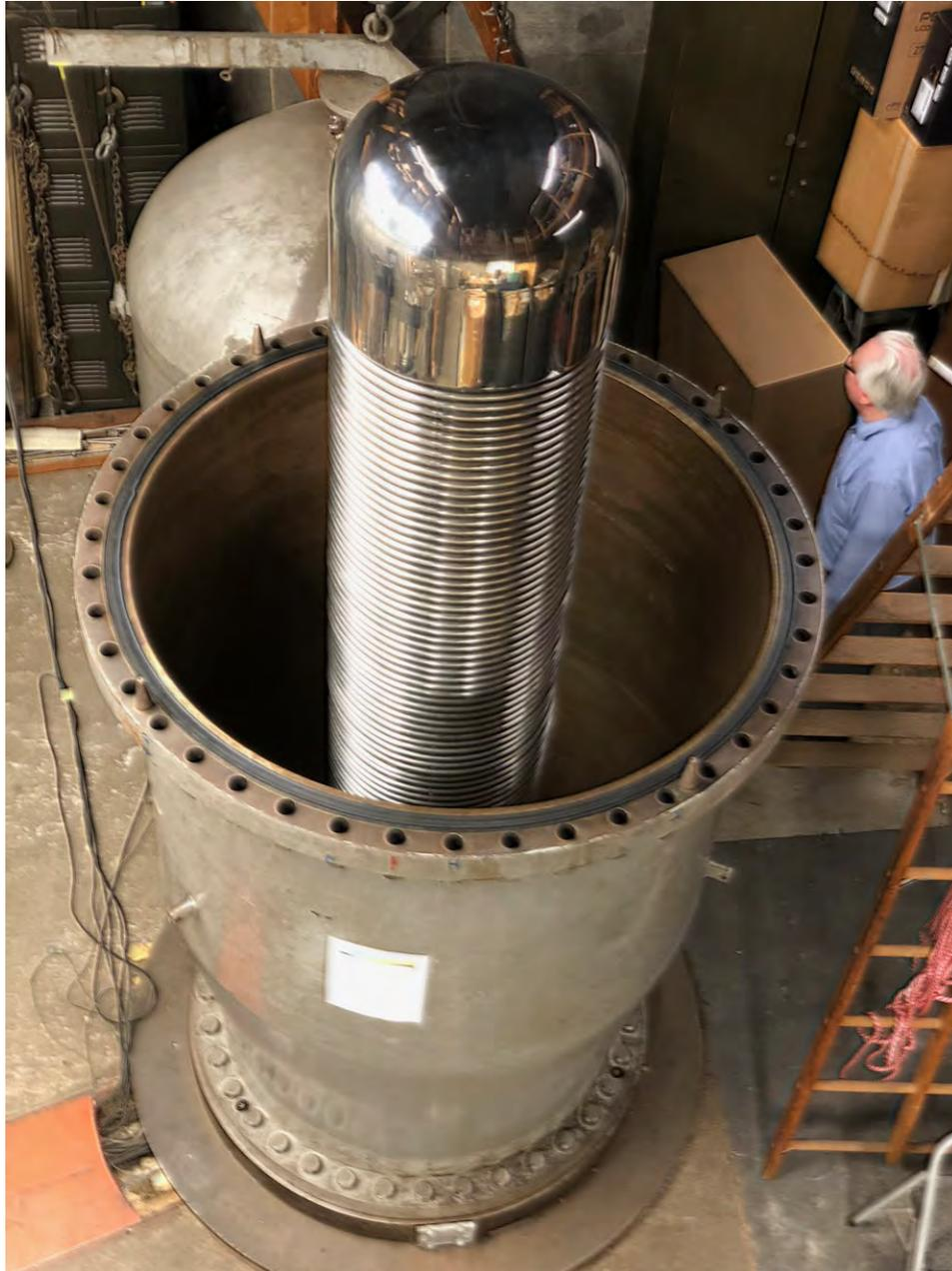
**Figure 3-5:** The acceleration column inside the tank.
