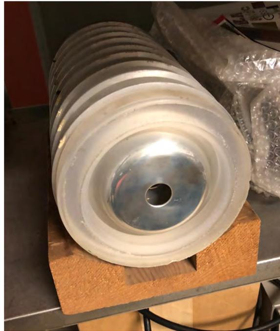
**Figure 3-4:** A set of electrodes similar to those inside the tank. This particular set is optimized for ion beams and contains curved electrodes. Those used for electron beams are flat.
