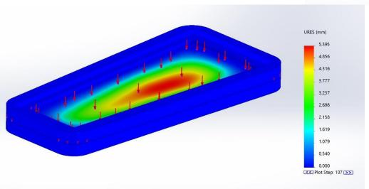
The analysis shows approx. 1/4 inch of displacement. The smaller window has less deflection.
