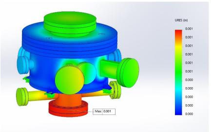
FEA of displacement is also very low (0.001"). No issues with target position when chamber is pumped down.
