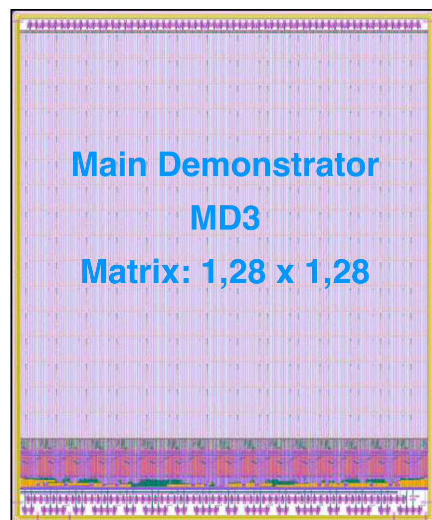
110 nm CMOS CIS technology, high-resistivity bulk, operated in full depletion mode
