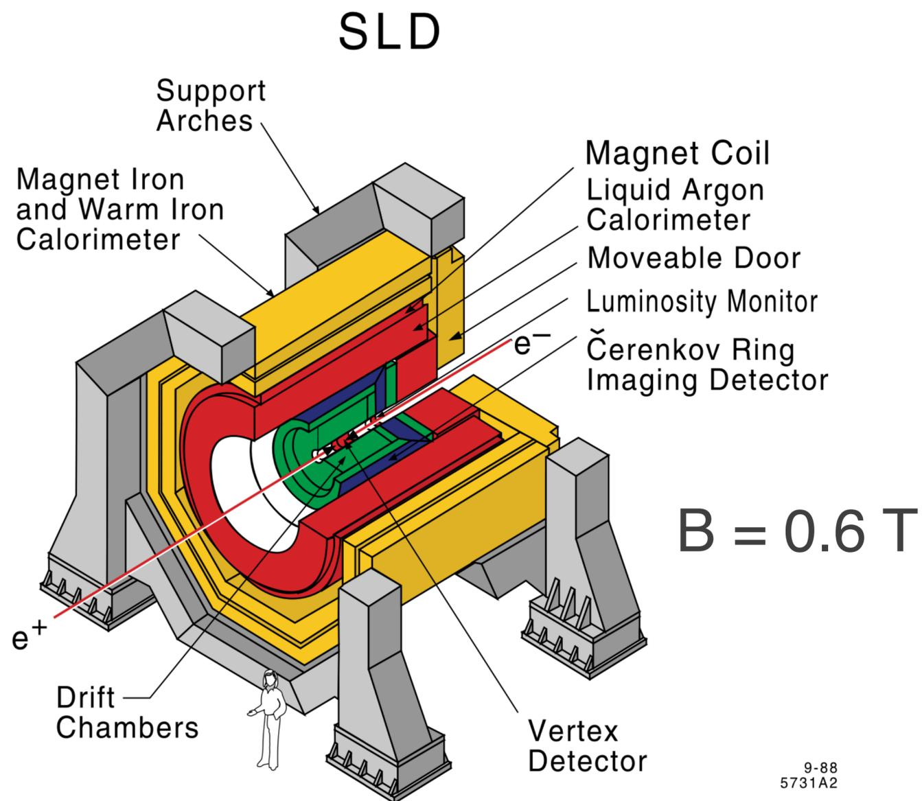
A Čerenkov Ring Imaging Detector combined with a drift chamber and vertex detector
