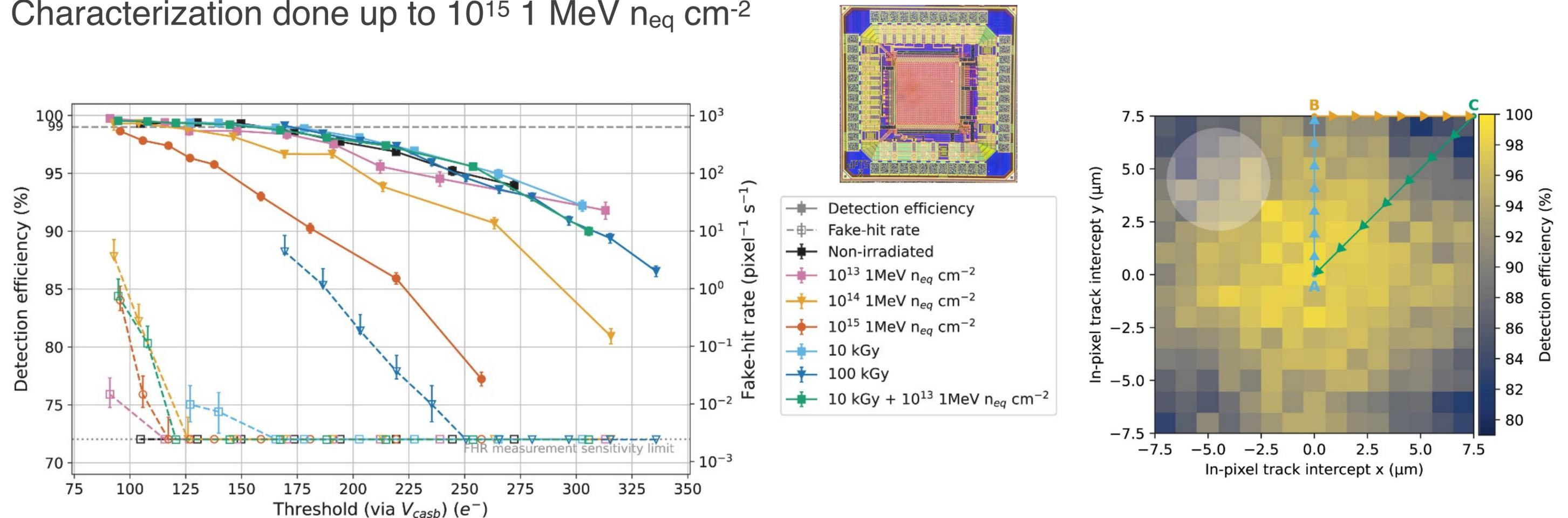
Digital pixel test structures implemented in a 65 nm CMOS process
