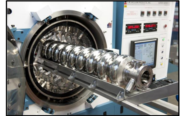
1.3 GHz 9-cell baking treatment
