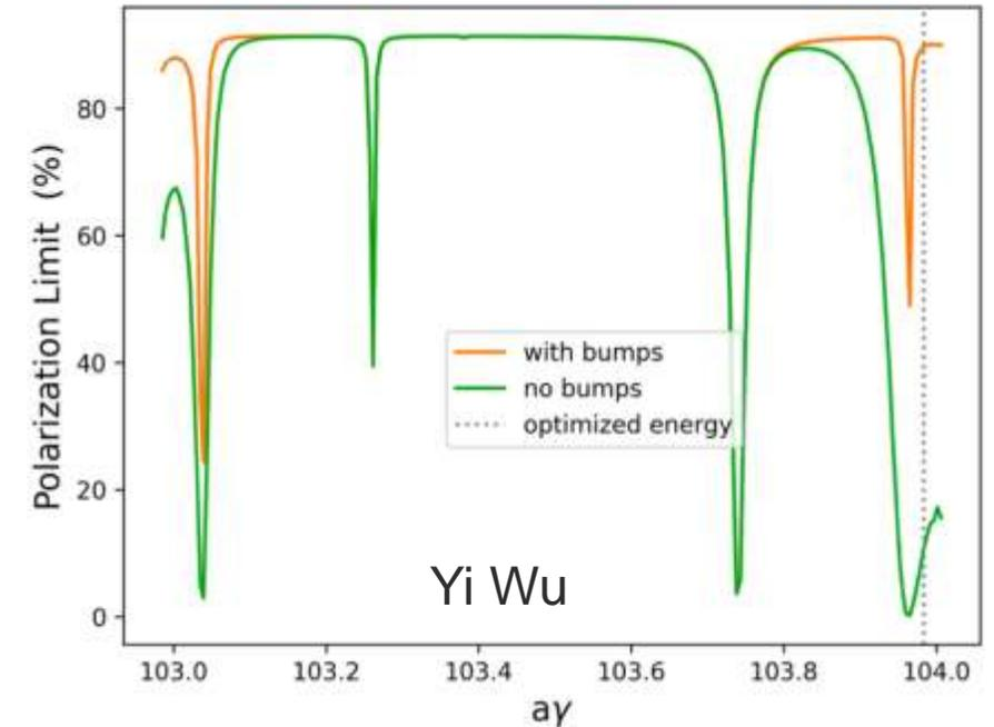
*First order energy scan with and without harmonic bumps optimized at 45.82 GeV ( $ay = 103.983$ ) using the Rossmannith-Schmidt scheme in V22 lattice*
