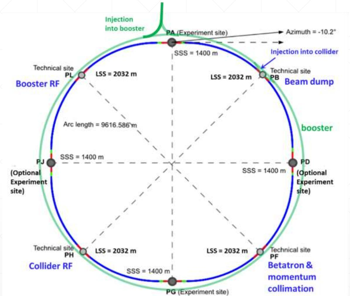
Optimised FCC-ee collider layout with 4 interaction points
